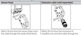
Within 30 mm from the connector of amplifier unit, wind the cable through the core three times and mount the ferrite core. mount the ferrite core.
